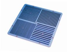
Four-quadrant bar phantoms offer precise determination of camera intrinsic resolution, collimator spatial resolution, field size and linearity.
