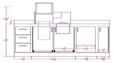
Cabinet Dimensions and Lead Thickness Can Be Customized To Your Specifications
